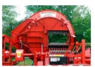
Hydraulically tilt the tub for easy access to grates and anvil for routine maintenance.
