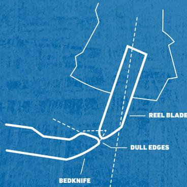
This profile drawing of the blades shows the result of wear. The leading edges are rounded and the angle of the bedknife has worn to match the circle created by the blade path. Rounded edges on the reel blades and bedknife will cause the grass blades to be pinched and torn rather than sheared off cleanly.
