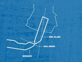
This profile drawing of the blades shows the result of wear. The leading edges are rounded and the angle of the bedknife has worn to match the circle created by the blade path. Rounded edges on the reel blades and bedknife will cause the grass blades to be pinched and torn rather than sheared off cleanly.
